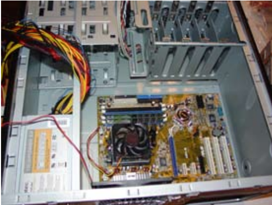
We installed the motherboard in the computer case, where we had already installed the power supply and an extra cooling fan. The video card was not yet in, and none of the cables from either the power supply or the case were connected, as you can see. Connecting all those cables, and figuring out where to connect them, took more time than anything else. Later on we installed the hard drive and DVD drive,
