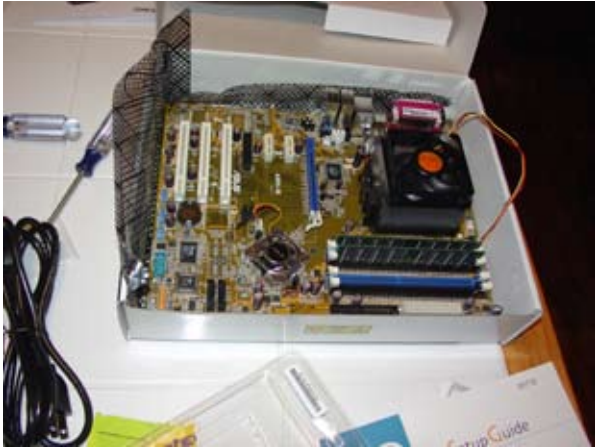
The motherboard is still in the box, and that is where we installed the CPU, the thermal grease, the cooling fan, and the memory. According to one web site, that method gave us more room to work. You can't see it in the picture, but we had the windows open to increase the humidity to decrease the probability of static electricity, which kills computers. Be sure to ground yourself well each time before touching the computer.
